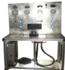
Servo Valve Test rig
