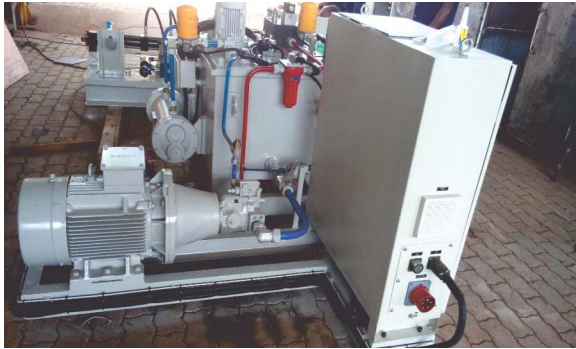
Hydraulic Power unit
