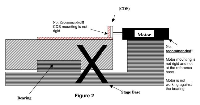
The motor should be mounted in such a way that the preload force is generated in the plane of the bearings, as shown in Figure 1. The bearings used with Nanomotion motors should be high quality linear or rotary bearings especially suitable for high precision applications. For linear applications, cross roller bearings are preferable, and air bearings are optimal. For low precision motion applications and those applications using actuators, lower cost ball bearing stages may be used.
