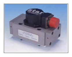
2-stage mechanical feedback Low mass, high band-width torque motor High spool drive forces Long life "Sapphire Technology" design High resolution, low hysteresis Rated flows 4 to 70 l/min at 70 bar Standard & High Response Internal pilot supply (4 port) ISO 4401 size 5
