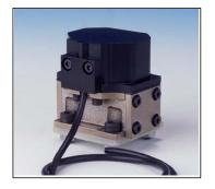
2-stage mechanical feedback (miniature) Low mass, high band-width torque motor High spool drive forces Long life "Sapphire Technology" design High resolution, low hysteresis Rated flows 2 to 7 l/min at 70 bar High Response Internal pilot supply (4 port)
