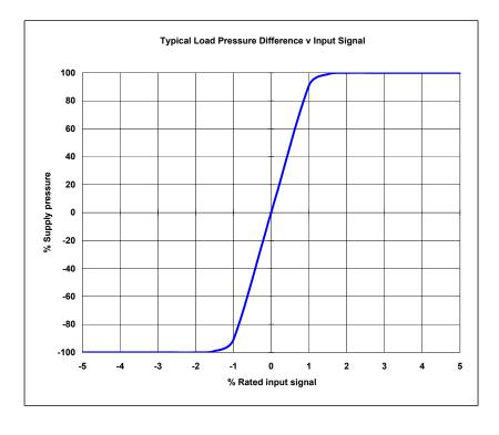
Pressure gain characteristic will vary with positive and negative lap conditions.
