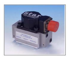
2-stage mechanical feedback Low mass, high band-width torque motor High spool drive forces Long life "Sapphire Technology" design High resolution, low hysteresis Rated flows 4 to 20 l/min at 70 bar Standard & High Response Internal pilot supply (4 port) ISO 10372 size 2
