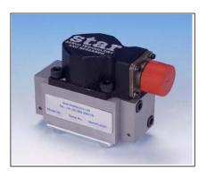
2-stage mechanical feedback Low mass, high band-width torque motor High spool drive forces Long life "Sapphire Technology" design High resolution, low hysteresis Rated flows 4 to 20 l/min at 70 bar Standard & High Response Internal pilot supply (4 port) ISO 4401 size 3
