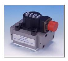
2-stage mechanical feedback Low mass, high band-width torque motor High spool drive forces Long life "Sapphire Technology" design High resolution, low hysteresis Rated flows 4 to 75 l/min at 70 bar Standard & High Response External pilot supply (5 port) ISO 10372 size 4
