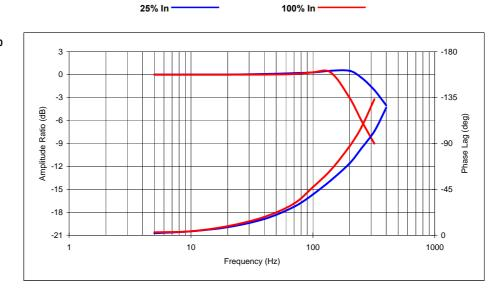
Typical performance curves optimised per 210 bar supply pressure, fluid viscosity 32 cSt at 40  $^{\rm o}{\rm C}$
