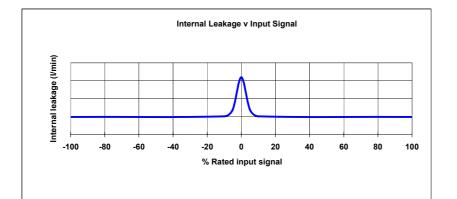
This comprises of both 1st stage flow (tare leakge) and the second stage null leakage.
