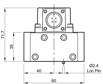
1. Suggested mounting bolts M8 x 60 long high tensile steel socket head cap screws.
