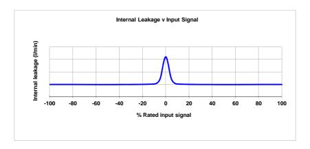
This comprises of both 1st stage flow (tare leakge) and the second stage null leakage.
