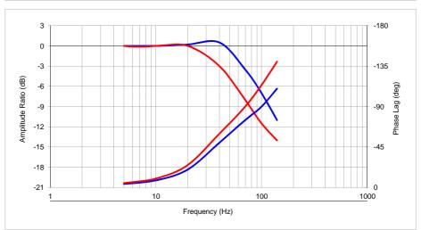
Typical performance curves optimised per 210 bar supply pressure, fluid viscosity 32 cSt at 40  $^{\rm o}$ C
