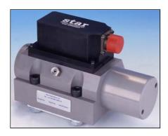
2-stage electric feedback, on board electronics Low mass, high band-width torque motor High spool drive forces Long life "Sapphire Technology" design Higher resolution, lower hysteresis Rated flows 95 to 230 l/min at 70 bar Higher frequency & step response Internal pilot supply (4 port) ISO 10372 size 6
