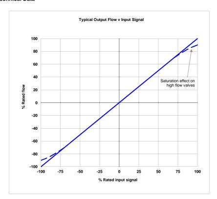
The flow tolerance for standard servovalves is ±10% of the rated flow at 100% rated input signal.
