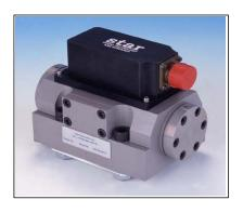
2-stage mechanical feedback Low mass, high band-width torque motor High spool drive forces Long life "Sapphire Technology" design High resolution, low hysteresis Rated flows 95 to 230 l/min at 70 bar External pilot supply (5 port) ISO 10372 size 6
