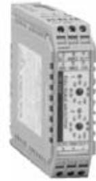
The VC2100 voltage-to-current converter transforms  $\pm 10V$  signals into current signals capable of driving hydraulic servo valves or similar loads. It also provides a convenient way to set the full scale current to match valve requirements, limit maximum current, or set optimum working ranges.
