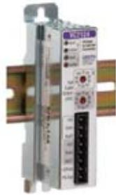
The VC2124 voltage-to-current converter transforms  $\pm 10V$  signals into current signals capable of driving hydraulic servo valves or similar loads. It also provides a convenient way to set the full scale current to match valve requirements, limit maximum current, or set optimum working ranges.
