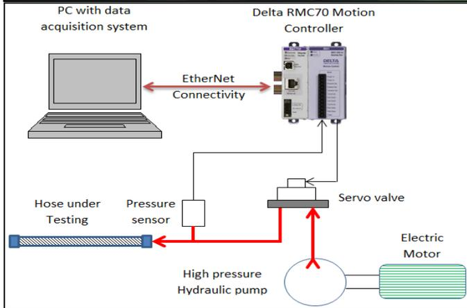
Impulse testing is one of the key predictions of hose life. Impulse testing involves the pressurizing or cycling of hose pressure, often times up to 140% of working pressure, at rates up to 1 to 2 cycle per second while the hose is held in either a 90° or 180° configuration. An impulse testing is a very good indicator of assembly robustness.
