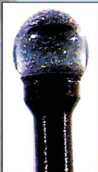
Sapphire at the end of feedback wire
