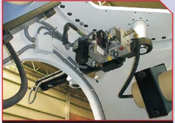
PITCH CONTROL AXIS WITH DDV ( DIRECT DRIVE VALVE)
